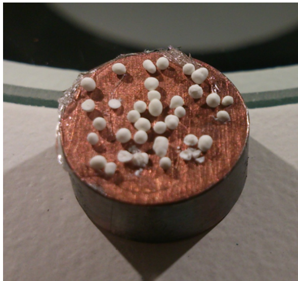
Figure 4.3: Beads of the W - ZrO_2 mounted on SEM-stub. Some of the beads are split in order to expose the inside.
