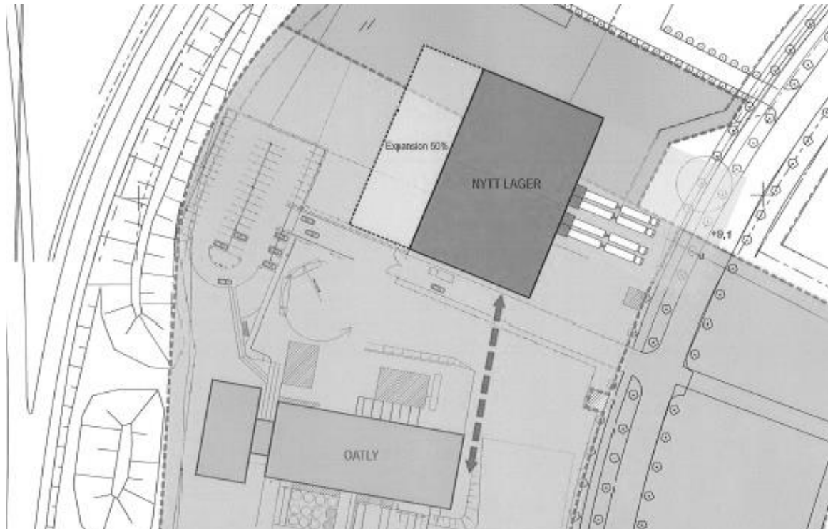
Figure 4.28. The Landskrona facility with the current warehouse is marked "NYTT LAGER" and the 50 % expansion. The building marked "OATLY" is the production facility.
