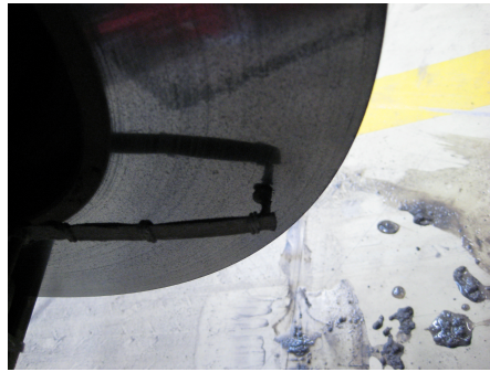
Figure 3.2 The outer temperature sensor on the disc brake.
