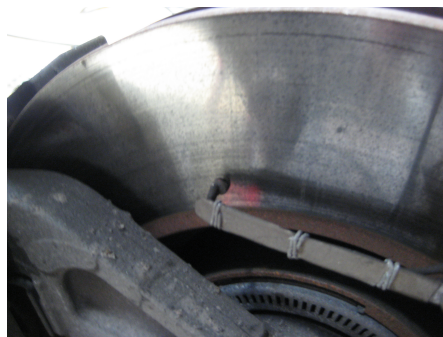
Figure 3.3 The inner temperature sensor on the disc brake.
