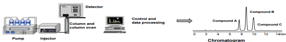
Figure 8. Main components of GPC/SEC equipment: pump, injector, column, detector and software (Image reproduced from http://polymer.ustc.edu.cn/xwxx_20/xw/201109/P020110906263097048536.pdf ) (41).
