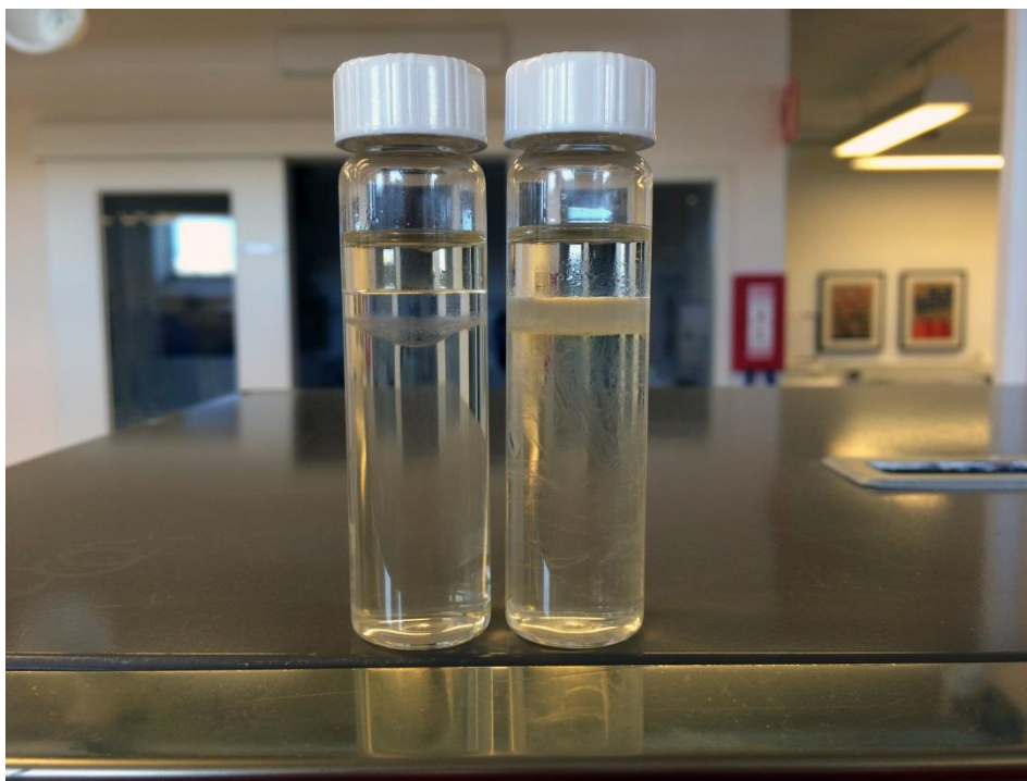
Figure 35. The formulations phase separates when put in a gelatine surface. A water rich phase forms closest the the gelatine surface and an oil rich phase floats on top.
