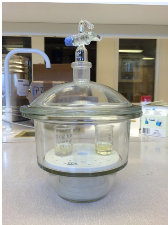
Figure 3. Picture of one of the exicators with the formulations in beakers inside.
