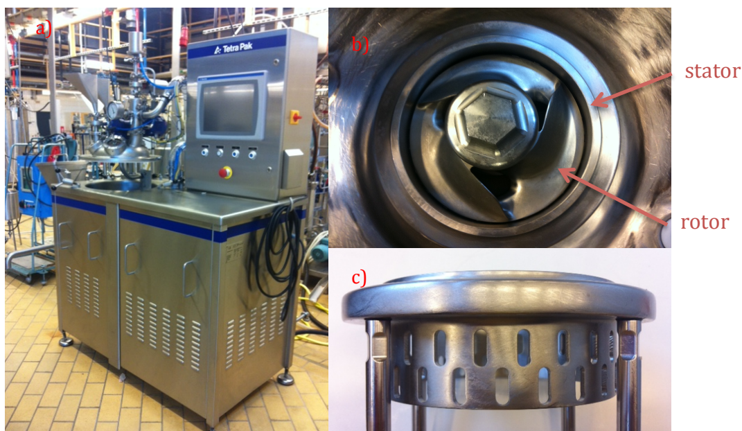
Figure 5. a) Tetra Almix B120-25VA, the vessel is located to the left of the mixer and the display to determine settings for the run is located to the right. b) (on top) The rotor head and stator seen from above. C) (bottom) The standard stator seen from the side.
