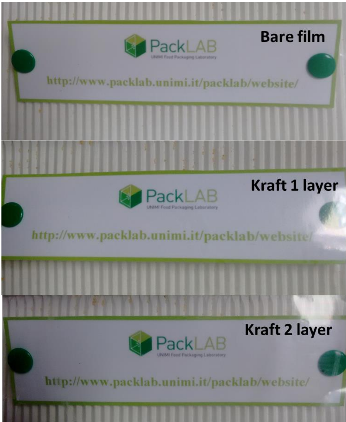
Figure 19. Text readability test (font 11 and font 6) on bare film, Kraft 1-layer, and Kraft 2-layer, showing that Kraft CNC coating (both 1-layer and 2-layer at 2.5%) has almost negligible influence to transparency.
