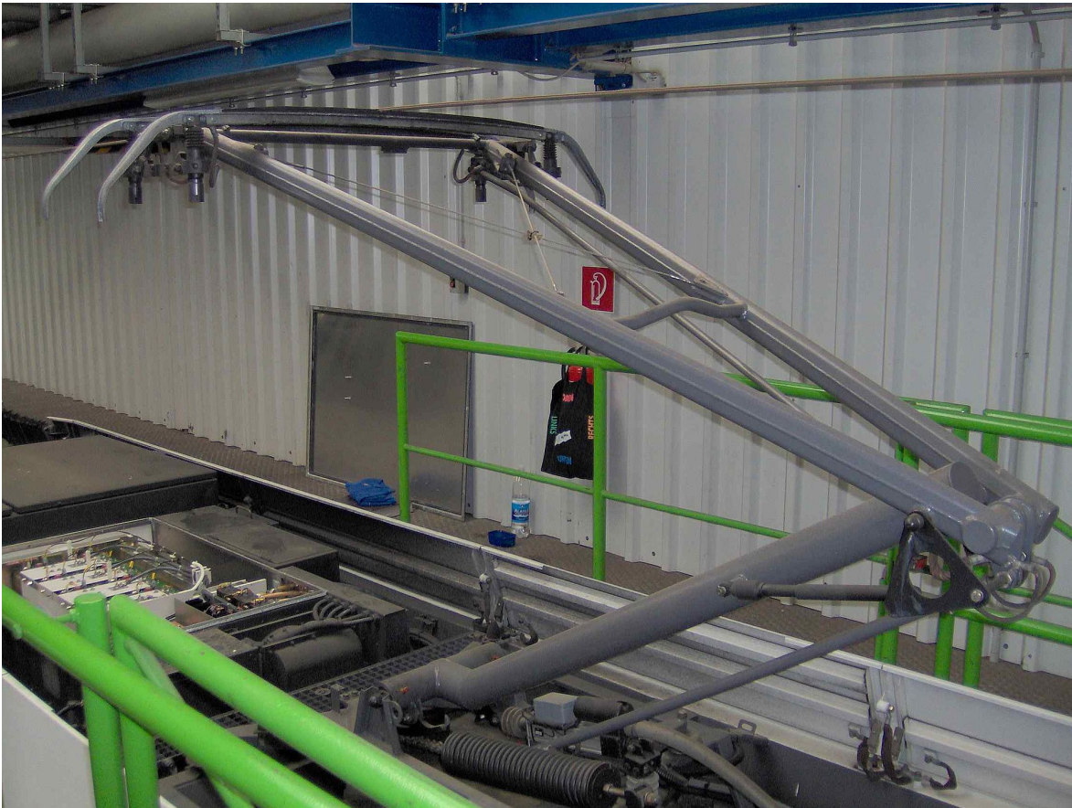
Figur 16 Strömavtagare/Pantograf (ProhibitOnions u.å).
