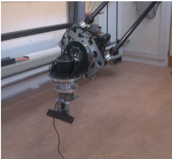
Fig. 10. L2 Gantry Tao Robot with mounted Xtion Asus Pro Live RGB-D camera.
