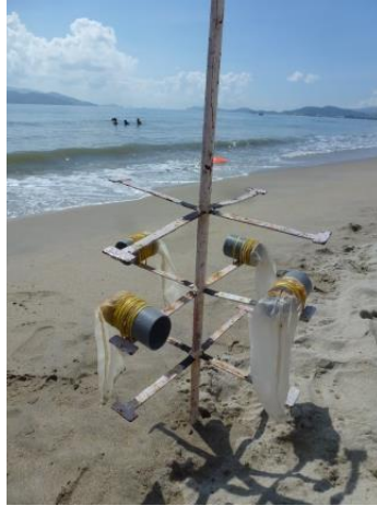
Figure 44. A Nagata sediment trap, developed by Yutaka Nagata, catches sediment transported in all cardinal directions in the nearshore zone .
