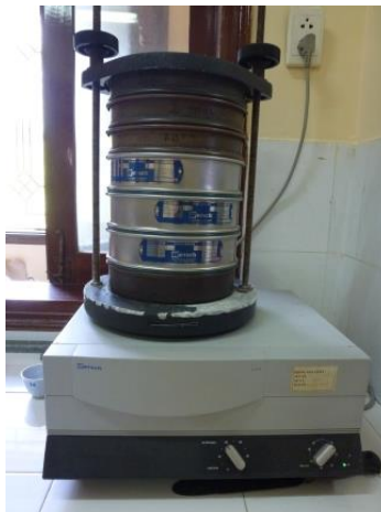
Figure 33. The instrumental setup used for sieving.
