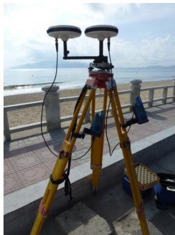
Figure 25. The levelling instrument with a ProMark 2 system from Ashtech was utilized to compile the coordinates for the present time shoreline and beach profiles.
