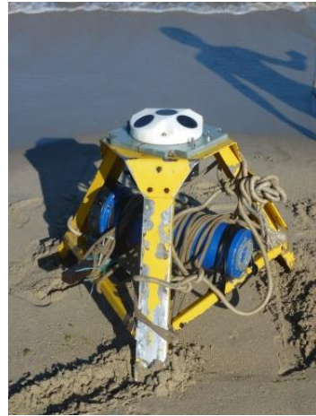
Figure 46. The Nortek AWAC (Acoustic Wave And Current Profiler) sensor used during the fieldtrip for gathering wave and current data.
