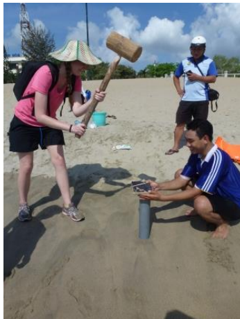
Figure 32. Sediment core samples were achieved by hammering down plastic pipes and pulling the cores up.
