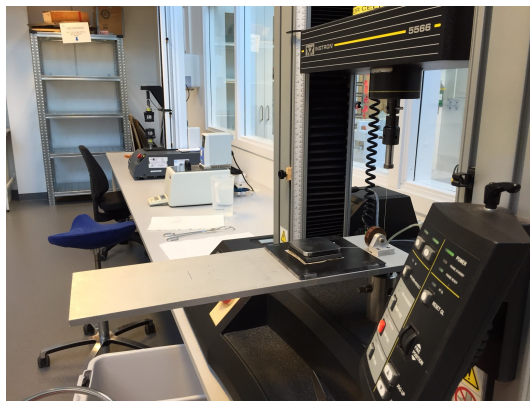
Figure 4.2 Measuring friction between a rubber sample and a carton sample. In the photo it is seen how the load cell pulls the sample along the table surface the table through a frictionless pulley with a nylon wire.
