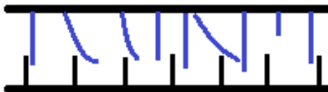
Figure 2.8 The contact mechanics between two bodies is theoretized as contact between elastic bristles. For simplicity the bristles of the lower body are thought of as rigid and the total elastical properties are therefore accounted for in the top body
