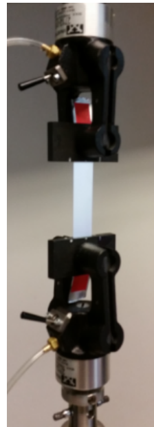
(d) Mounted sample, no tape outside of the fastened grips
