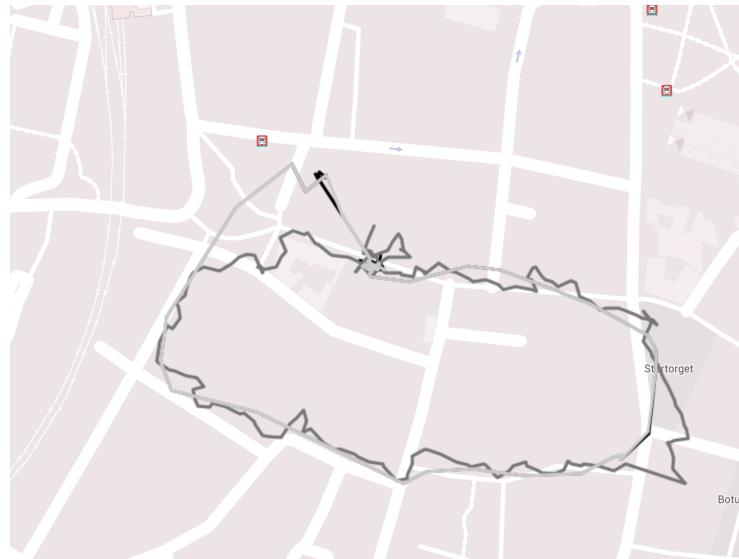
Figure 5.9: Black - All multilaterated positions, Light gray - unnecessary measurements removed, dark gray - MyTracks path.
