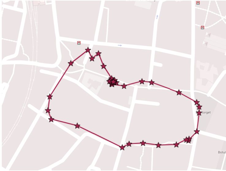
Figure 5.7: Estimated positions with our proposed localization algorithm. 213 unnecessary position estimates removed.
