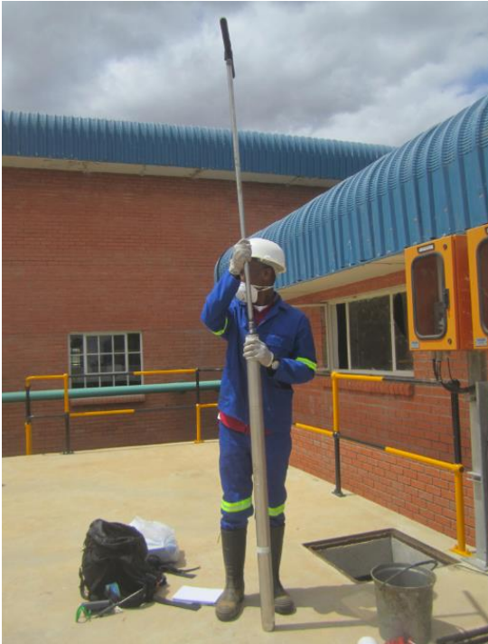
Figure 2.2 Sludge sampling from the buffer tank with the instrument Multi Stage Sludge Sampler.
