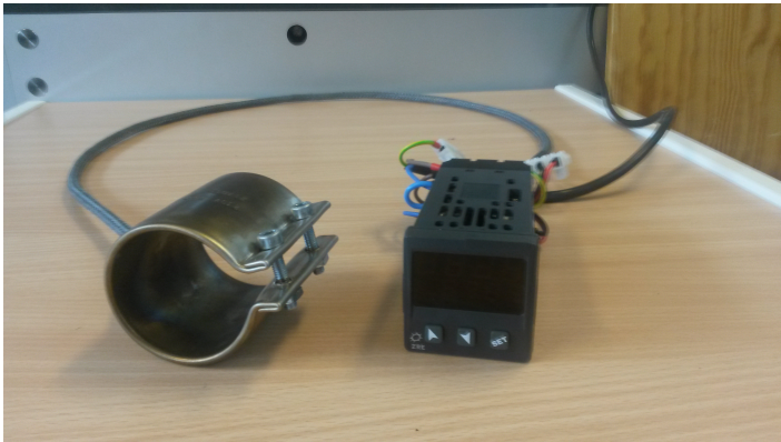
Figure 4.12 Heater band and temperature controller.
