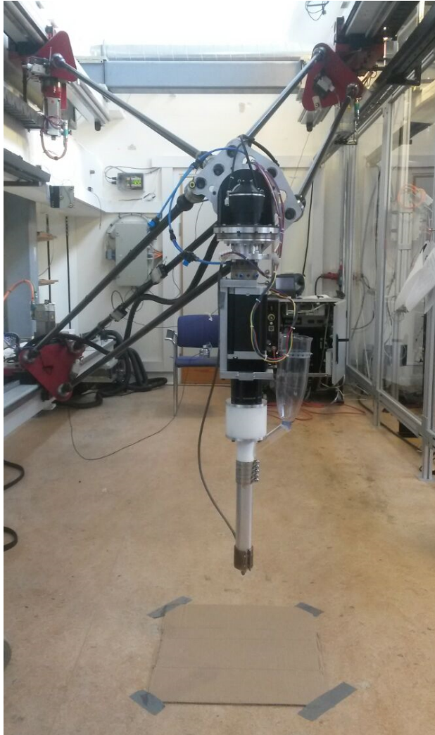
Figure 5.9 The 3D printer head prototype mounted on the L2 robot in the Robot Lab at LTH.
