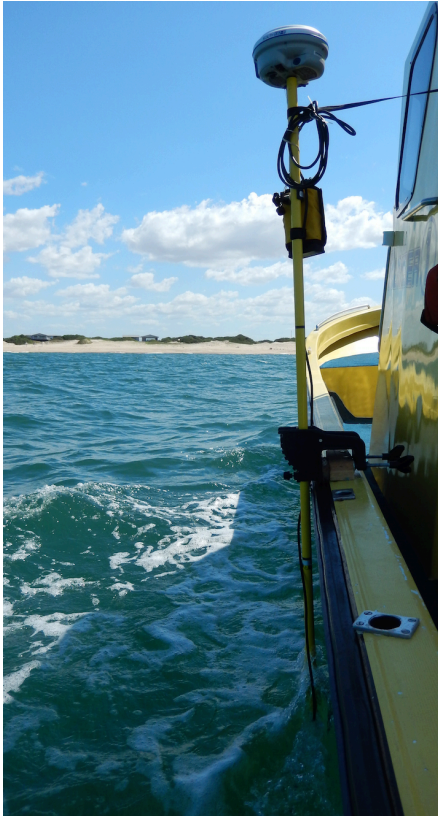
Figure 22. Echo sounder used during field investigations.
