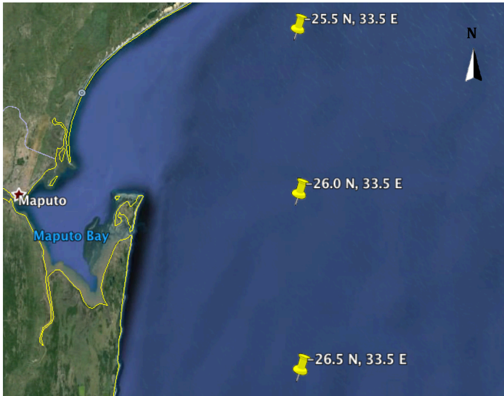
Figure 42. Three possible GPS positions for wave data extraction. The latitudinal distance between each 0.5^\circ is approximately 55km. From analysis of wave direction and topography -26.0 N, 33.5 E was chosen as the coordinate to extract the data from.
