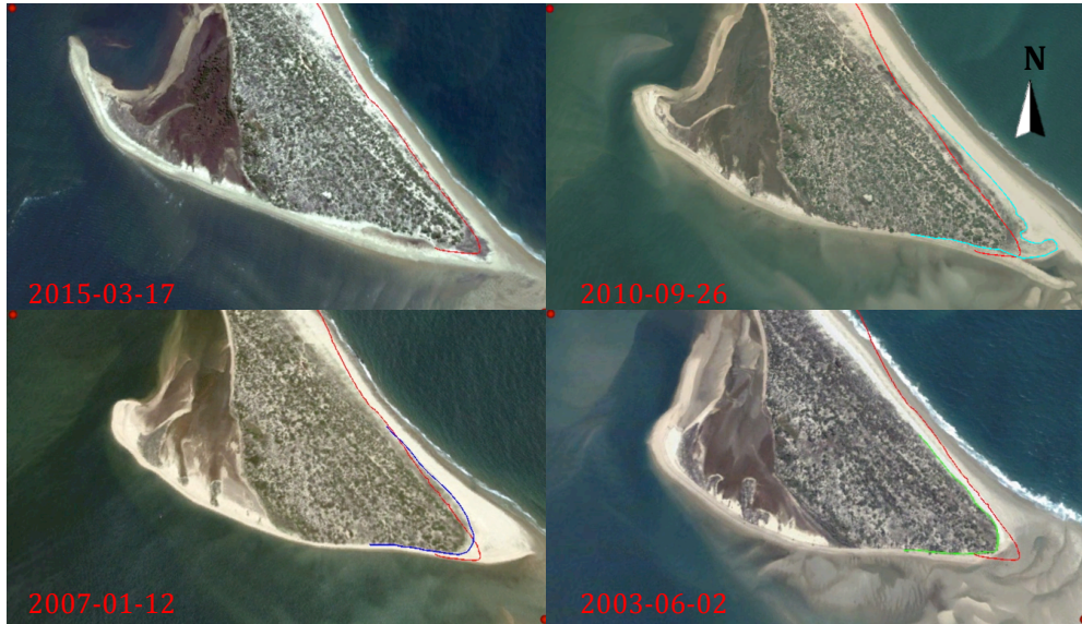
Figure 40. Surveyed shoreline position (2015-03-17) together with historical shoreline positions of the tip of Macaneta spit, displayed on old satellite images (Google Earth, 2014). From the top left to lower right: Surveyed shoreline printed on satellite image from 2014-08-30, Surveyed shoreline together with shoreline position from 2010-09-26, surveyed shoreline and shoreline position of 2007-01-12 and finally surveyed shoreline and shoreline position from 2003-06-02. All images are captured at an altitude of 1.32km above MSWL.
