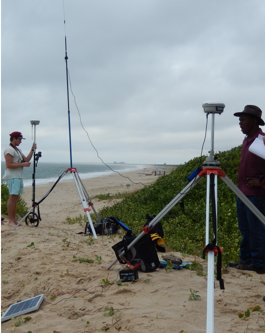
Figure 21. Differential GPS instruments used during the field survey. To the left the rover unit on wheel, to the right the base station and in the center an external antenna connected to the base station.
