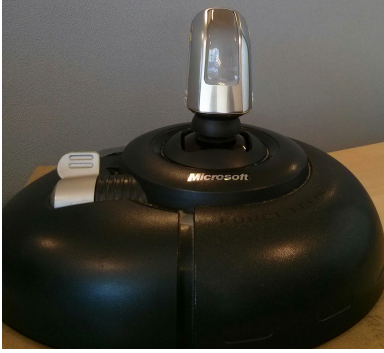
Figure 3: The chosen joystick was a Microsoft Sidewinder Force Feedback 2. The knob was changed by the Volvo XC90 gearstick, buttons were removed and the power was doubled.
