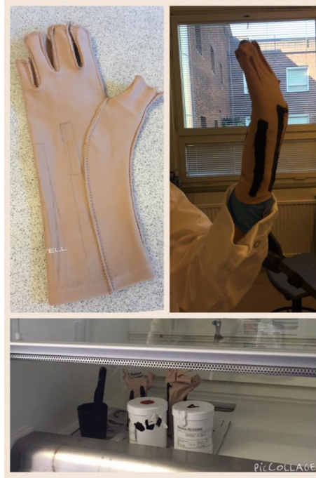
Figure 16: Top left: Pre painted compression glove, top right: painting the glove, bottom: Overnight curing in a fume.
