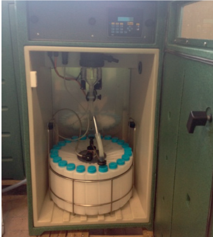
Figure 4.1. Automatic wastewater sampler used for the sampling of influent and effluent wastewater. Both time proportional and daily flow proportional samples were taken during the project period.
