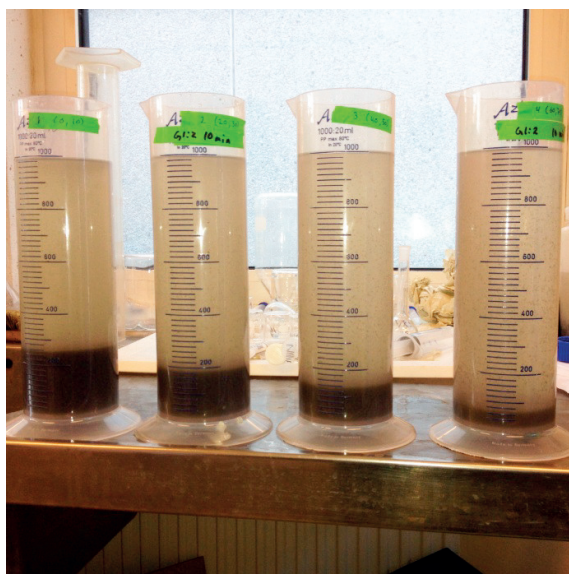
Figure 4.6. Principle for ZSV tests. Mixed liquor was mixed with tap water and let to settle in 1000 mL measuring cylinders. The picture shows four such cylinders shortly after the tests. The difference in dilution is indicated from the sludge volume at the bottom of the cylinders.
