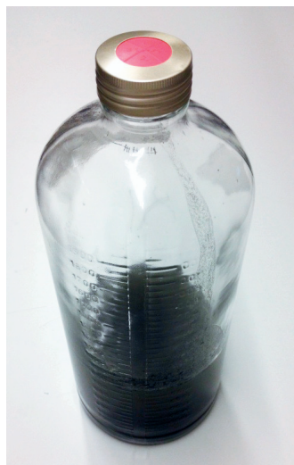
Figure 4.7. Glass flask reactor for methane production, equipped with a pressure tight rubber septum secured with a metallic lock. The depicted reactor contains a mixture of inoculum, tap water and WAS.
