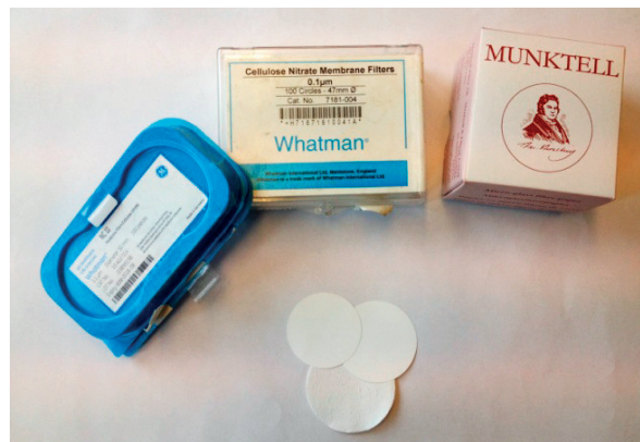
Figure 4.3. The two types of 0.1 \mu\text{m} cellulose membranes and the 1.6 \mu\text{m} glass filter paper used for filtration analysis.
