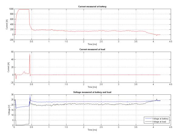
Figure 21: Currents and voltages typically appearing when squeezing a cable. The pattern was repeated when shaking the cable lightly. It corresponds to a short-circuit to ground during a limited time.
