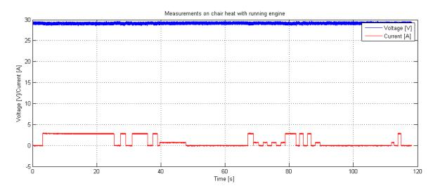
Figure 12: Voltage and current measured at the chair heating fuse
