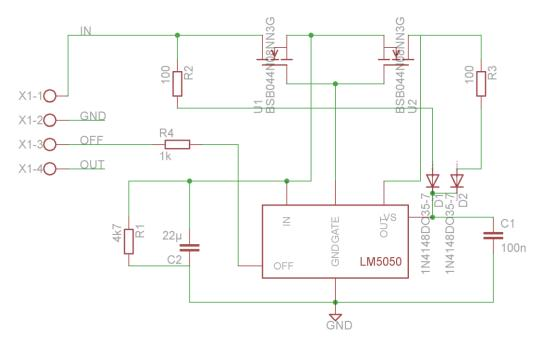
Figure 35: Anti-serial MOSFETs with LM5050 drive circuit. A solution proposed by Jan Hellgren, RECU.
