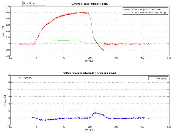
Figure 34: Short circuit testing of BTS555
