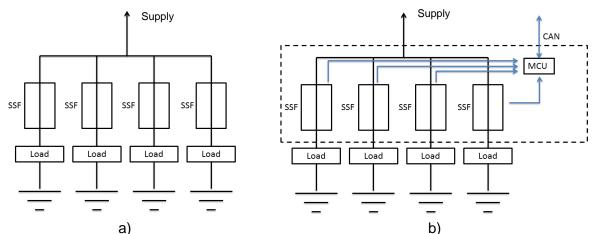
Figure 2: Principle structure for a) individual SSF units and b) multiple SSF units within the same SSF system and physical unit
