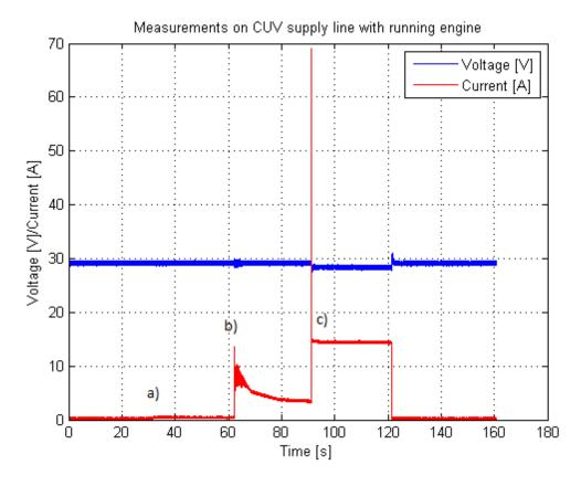
Figure 14: Voltage and current measured at CUV point of connection. Parking light switched on at a), dipped beam at b) and main beam at c)
