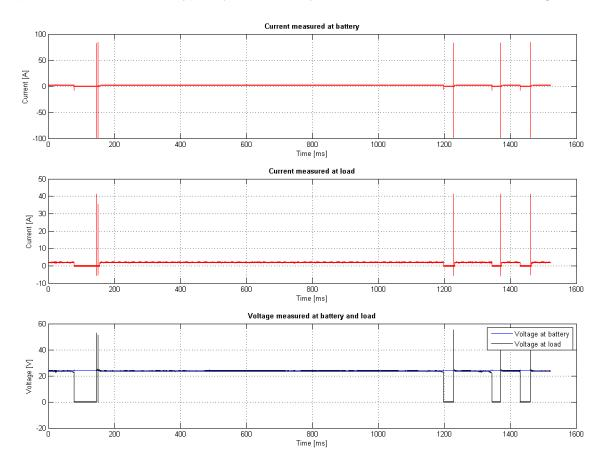
Figure 23: Currents and voltages measured when exposing a cable to bending
