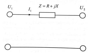
Figure 9: Short length cable model [23]
