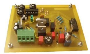
Figure 1: The Active Fuse System prototype built by Sjöberg and Steen in 2008 [2]
