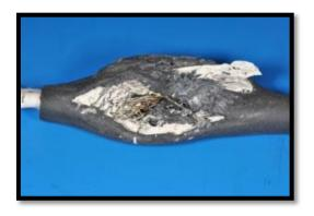
Figure 20: Cable after squeezing, 1 of 14 samples
