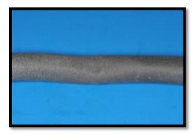
Figure 22: Cable after bending simulation, 1 of 5 samples
