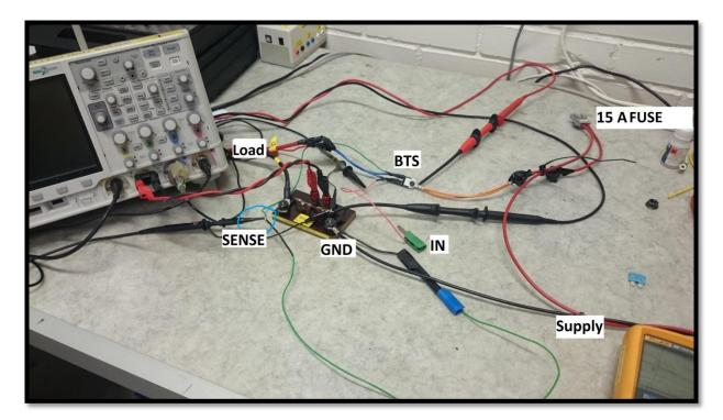
Figure 33: Setup for evaluating the BTS555
