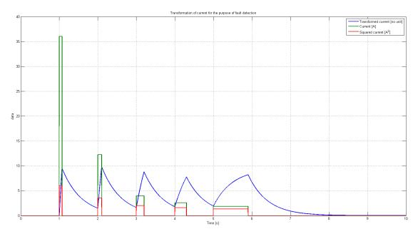
Figure 31: Transform of current test pulses according to ISO 8820-3
