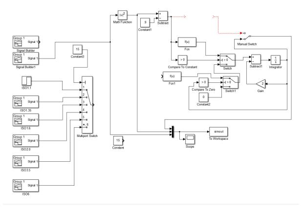
Figure 30: Experiment model for imitating the tripping scheme outlined in ISO 8820-3
