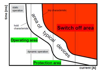
Figure 8: Internal tripping characteristic for a PROFET [22]
