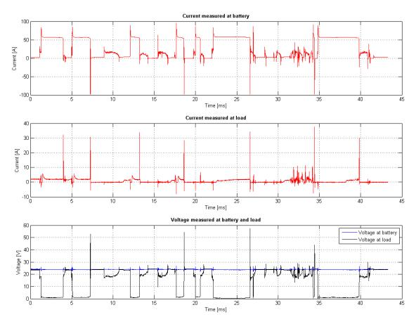
Figure 25: Currents and voltages measured during cutting-simulations
