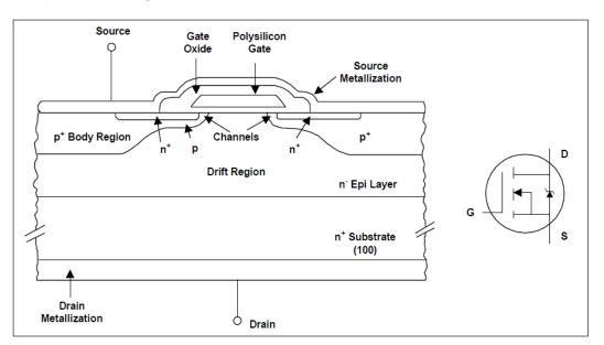
Figure 3: Structure and symbol of the n-channel MOSFET [10]
