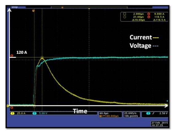
Figure 27: Current and voltage measurement performed on a component with severe inrush current and bypassed fuse
