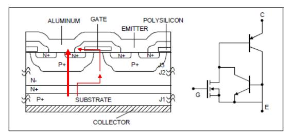
Figure 4: The IGBT structure and equivalent schematic [6]
