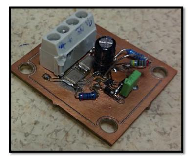
Figure 36: Circuit for evaluating anti-serial MOSFETs
