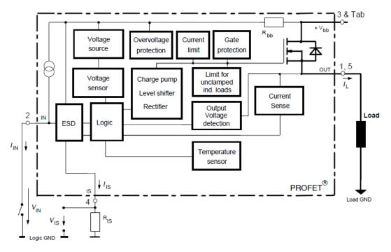
Figure 7: Schematic functional diagram of the Infineon BTS555 [21]
