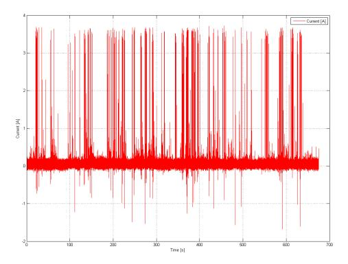
Figure 17: Current measured at the VGT
