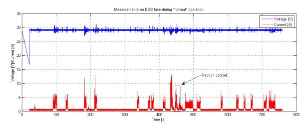
Figure 15: Voltage and current measured at EBS fuse
