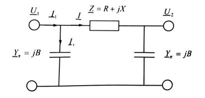
Figure 10: Medium length cable model [23]
