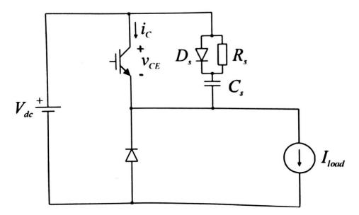
Figure 5: An example of a snubber circuit [6]
