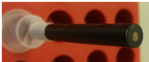
Figure 4.10: The image shows one of the two identical gold electrodes used during all the electrochemical measurements. Gold nanoparticles have been dropped on the gold surface and let to dry.
