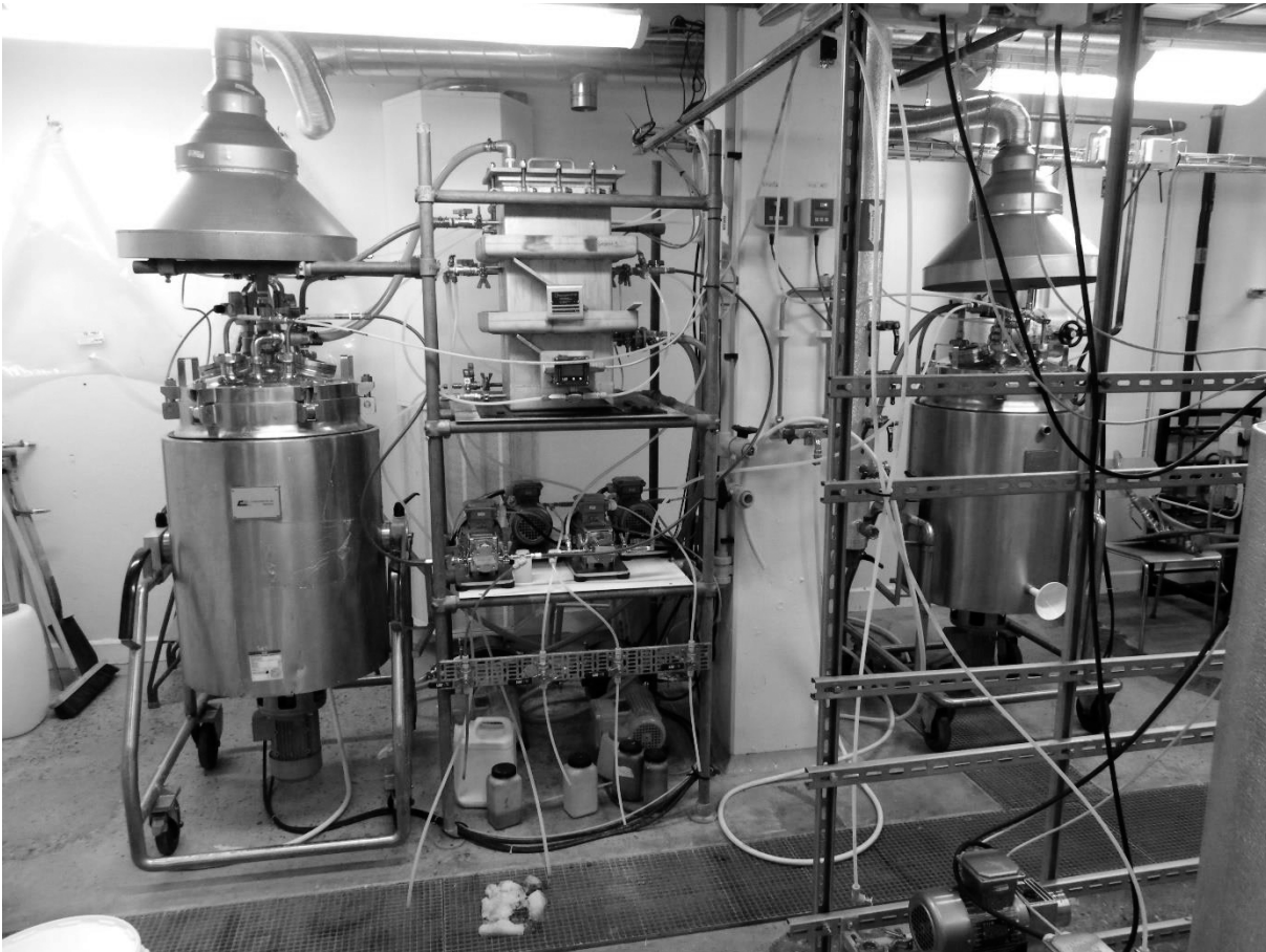
Figure 3-2. Image from all the system except substrate tanks. Reactor 1 (left), 2 (right), membrane filtration unit and filtration and biogas pumps (center).
