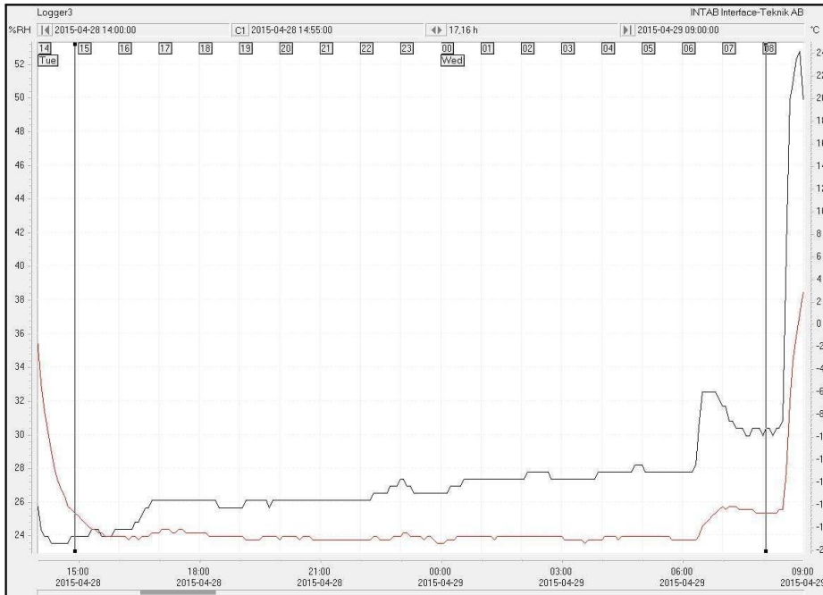
Diagram 3, logger 3 - red curve is temperature and black curve is humidity.
