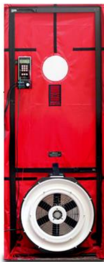
Figur 4.1: Blower Door. ( laminair-ab.com )
