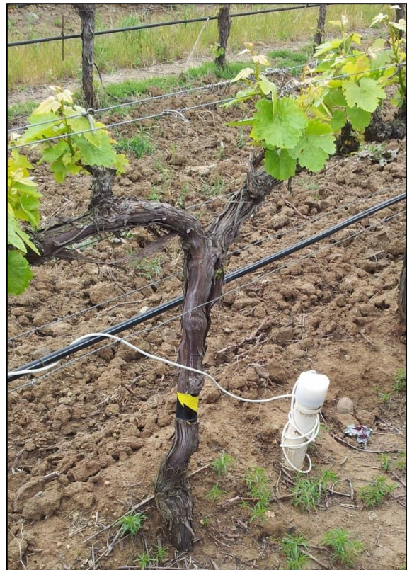
Picture 1: Soil probe connected to Wi-Fi readout transmitter.
