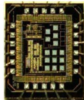
Fig. 2. RF CMOS transceiver at 433 MHz (1.6 mm×1.5 mm size dimensions) fabricated in CMOS 0.7 μm.
