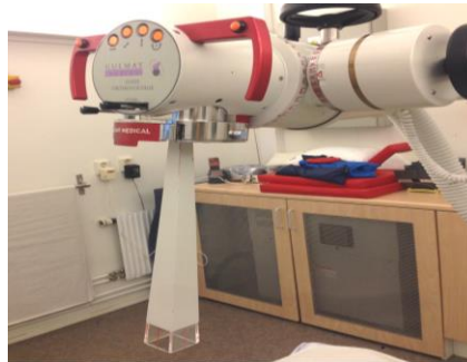
Figure 4: The Gulmay Medical x-ray unit with inserted applicator 4\times 4\text{ cm}^2 .
