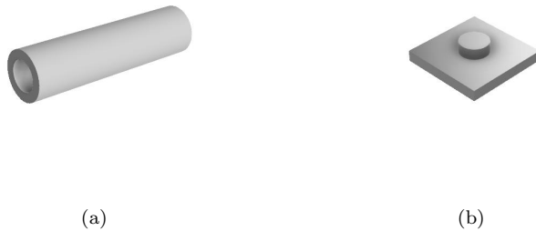
Figure 3: (a) The cylinder to cast the cylindrical part. (b) The base plate for the cylinder to stop the PVA mixture to leak out.
