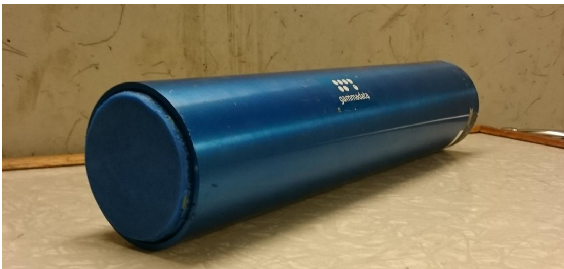
Figure 13. NaI(Tl) detector in aluminium rod with the front end cap removed.
