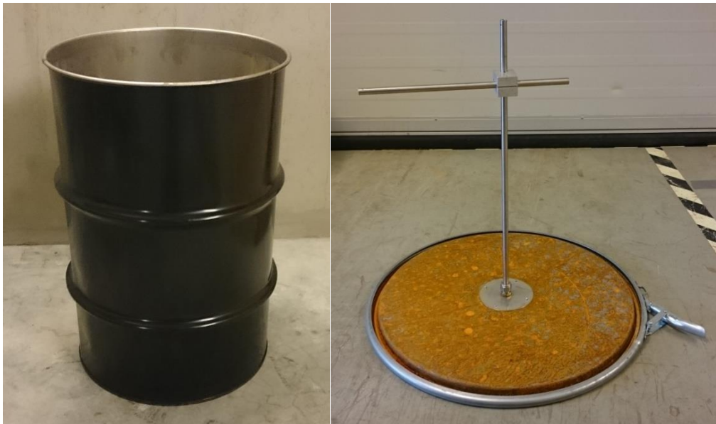
Figure 6. To the left a steel barrel with inside height 700 mm, inside diameter 470 mm and wall thickness 0.7 mm. The image to the right depicts a lid with aluminium rods used to place the sources at the first two setups.
