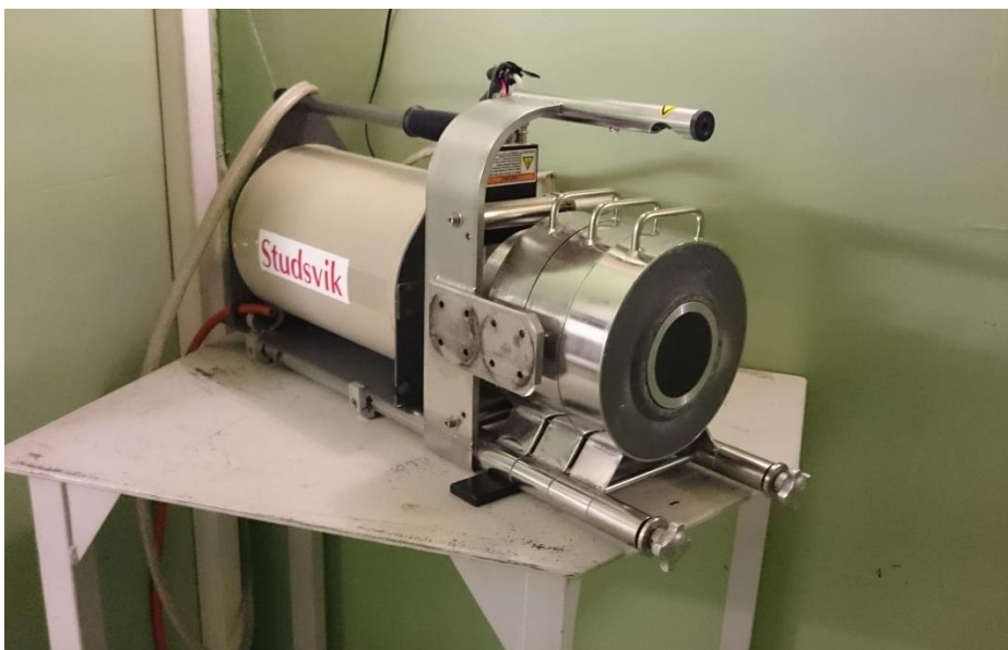
Figure 11. The system setup at “R0-A”, with the p-type HPGe detector with relative efficiency 48 % complete with cryostat and lead collimation.
