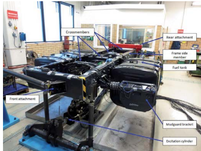
Figure 4: Overview of the experimental setup including a brief description of the components.
