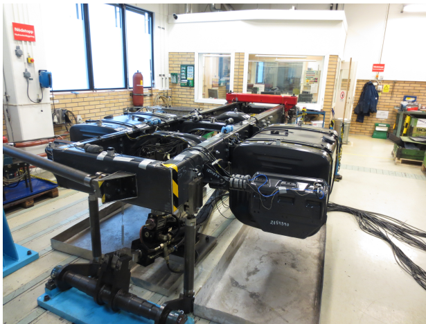
Figure 1: The experimental setup, consisting of a heavy vehicle chassis frame with a number of mounted components.
