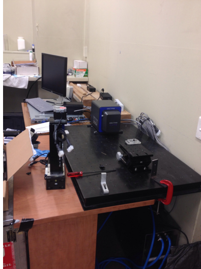
Figure 19: Preparing for a quantum efficiency measurement. The PILATUS3 CdTe with shield on is visible on the optical bench, along with the stage and perspex vial holder used to keep the vial with source in place. Lead shielding not in place at this point.
