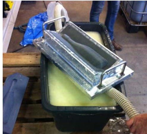
Figure 3.5 The aluminum tool covered with a fine mesh separating water and pulp.
