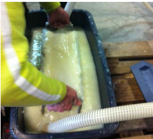
Figure 3.6 The tool is dipped into the pulp in order to create a mold.
