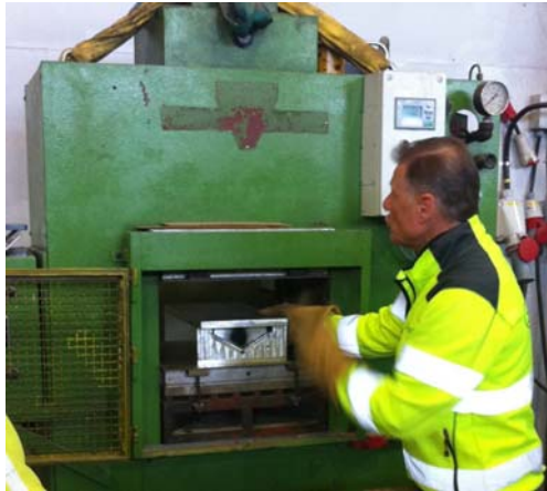
Figure 3.10 Heat pressing, the mold is placed between the two tools and activation occur.
