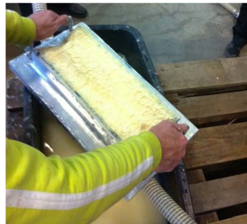
Figure 3.7 A mold is created and fixated on the tool with vacuum.
