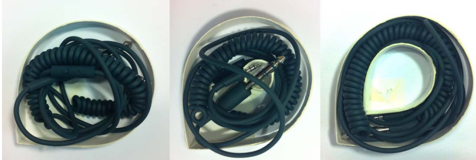
Figure 7.14 Outcome after prototyping brainstorming about how to store the detached cable in the package. From left to right; prototype with only one cavity, prototype with attachment for cable and prototype with an elevation in the middle.
