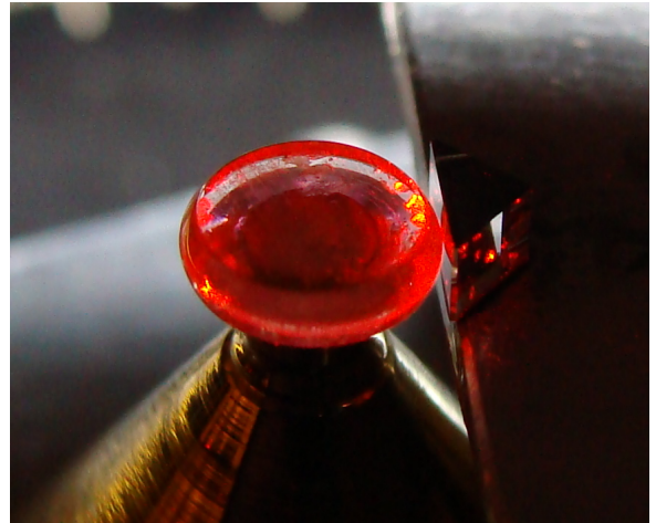
Figure 31: A photograph of the Whispering Gallery Mode Resonator with light coupled into it. The red 'glow' shows the fluorescence from the Praseodymium ions, due to the interaction with in-coupled light.
