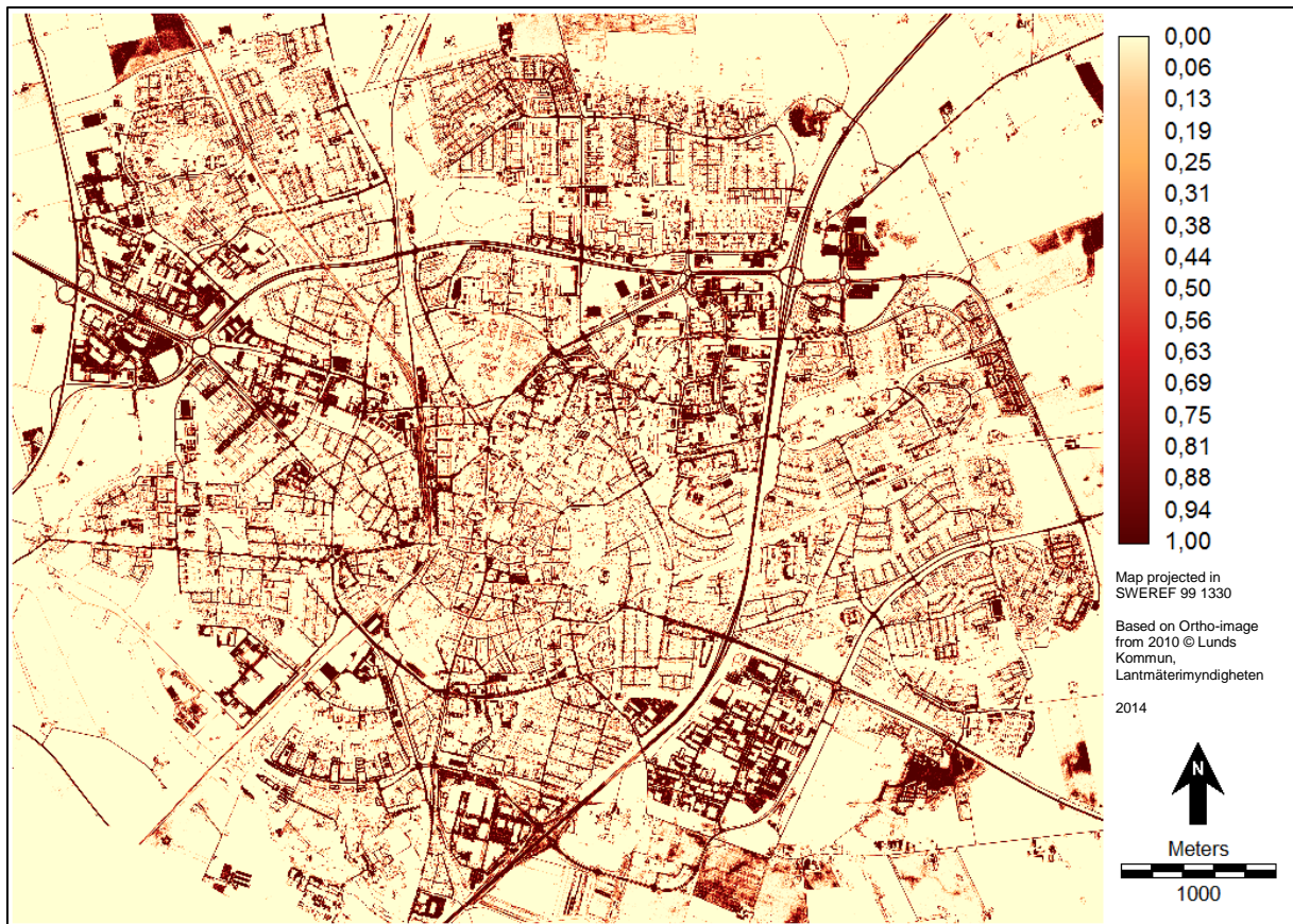
Figure 11 The percentage impervious area within the study area. The range of imperviousness is shown as a proportion representing %. Buildings have been extracted from the impervious areas as these are assumed pervious.
