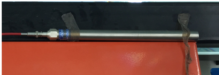
Figure 2.8: {}^3\text{He} Proportional Counter. Top-view. Photograph by author.
