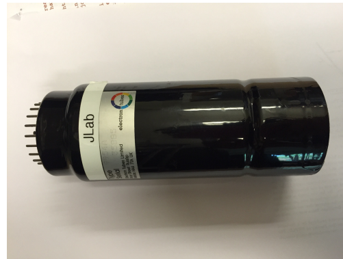
Figure 2.5: Photomultiplier Tube. (a) generic illustration; (b) photograph. Figure from Ref. [17]. Photograph by author.
