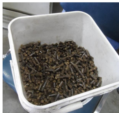
Figure 5-4: Pellets produced by blending woodchips and shredded cattail
