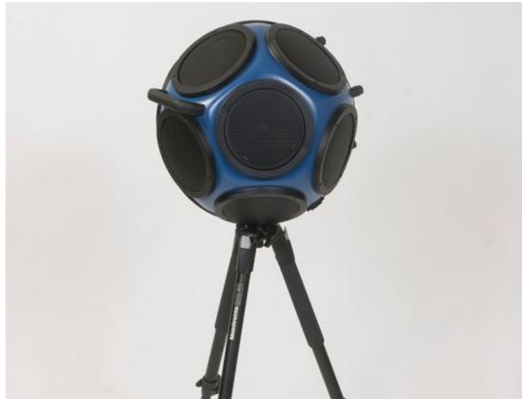
(a) The Norsonic Nor 270 dodecahedron speaker used to for background noise simulation.
