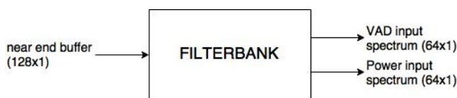
Figure 4.4: Block figure of the 128-point FFT analysis filter bank with its in and outputs.
