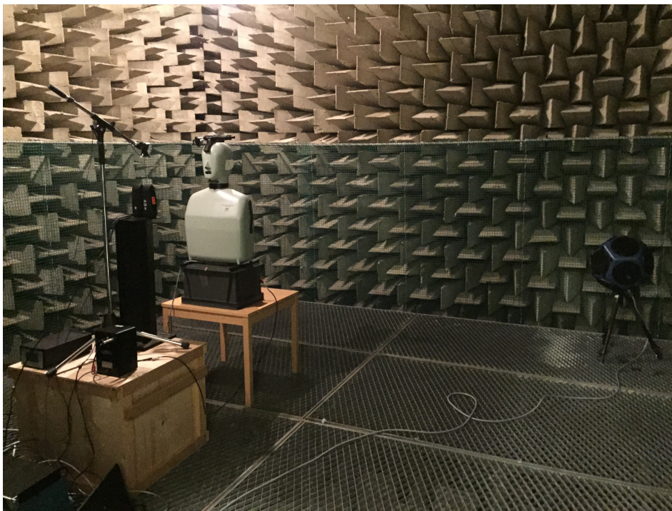
Figure 4.21: Anechoic chamber with all equipment used as described in this chapter.
