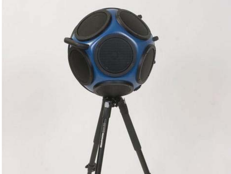
(a) The Norsonic Nor 270 dodecahedron speaker used to for background noise simulation.
