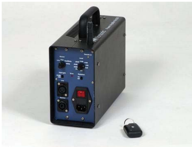
(b) Nor 280 Power Amplifier used for the Nor 270 speaker.
