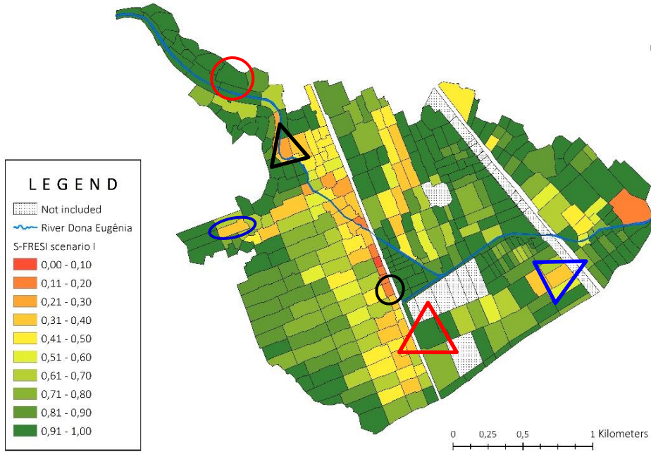
Figure 7.13. S-FRESI for scenario I, present time without flood control modifications. Red markings show areas with low flood levels, blue medium flood levels and black high flood levels. The circles mark areas with higher income and triangles mark areas with lower income.
