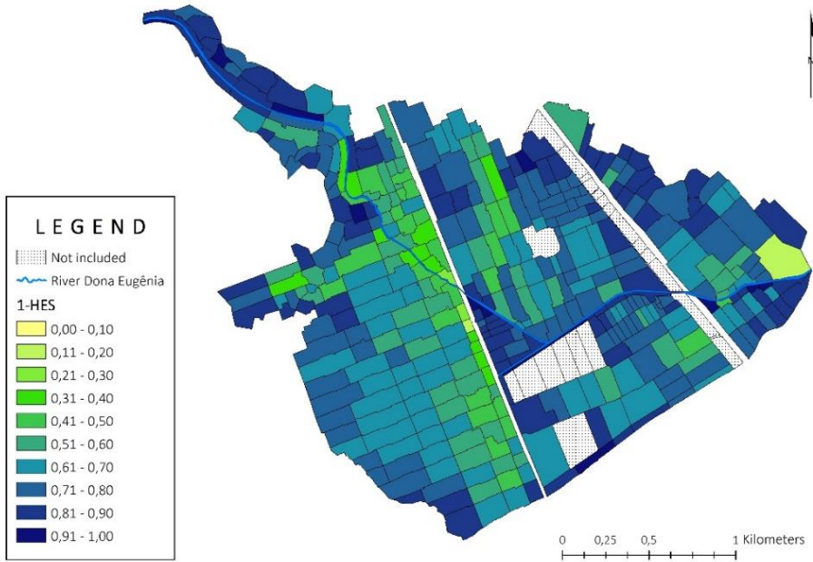
Figure 7.10 Combination of Hazard, exposure and susceptibility as it is in S-FRESI.
