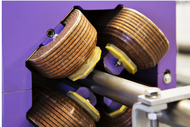
Figure 5: A quadrupole magnet installed at the MAX IV Laboratory 3 GeV storage ring. [3]
