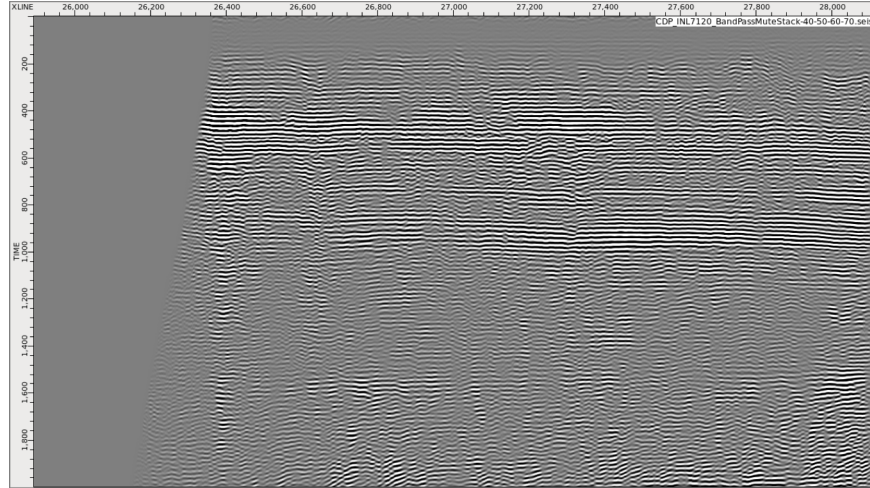
Figure 5.18: The inline acquired with narrow azimuth 3D streamers and high definition processed is here frequency filtered and passed for 40-70 Hz. It is also muted and stacked. X-axis is the CMP numbering with equal spacing. Y-axis is the two-way-time expressed in seconds.
