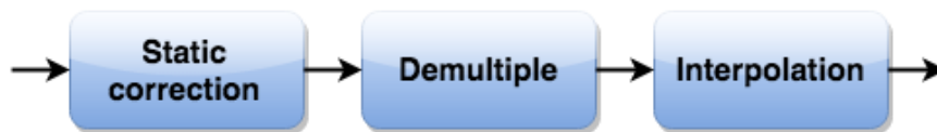
Figure 3.3: Crucial part of reprocessing sequence for high definition flow of conventionally acquired 3D data. For static correction see appendix A. The principles of demultiple are explained in 2.4.2. The nature of interpolation is expected to be known but how the interpolation is effecting the imaging is explained in this section.
