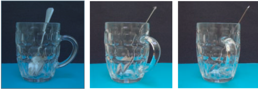
Figure 2.8: Illustration the meaning of azimuth. Image changes with the relation of direction between the spoon and irregularity of the glass. From the left the spoon is fully visible, distorted in the middle and invisible to the right. (Brice et al., 2013)
