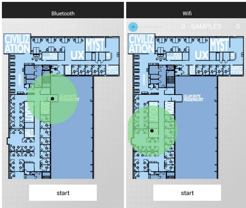
Fig. 31. This figure presents the creation of a reference area on the smartphone application. This done by using Bluetooth proximity, to the left, or by using Wi-Fi fingerprints, to the right.
