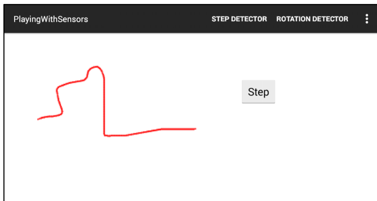
Fig. 38. This figure shows a pedestrian dead reckoning (PDR) solution based on gyroscope and accelerometer. It recognizes when the user has taken a step and the smartphones current angle. The step button simulates a step. The red curve represents the path which the smartphone experienced while the user walked around. The white area represents the floor of a room.
