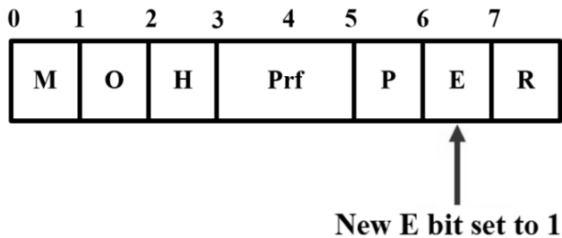
Fig. 18. The new E bit added to the RA flag field [2]
