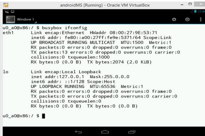
Fig.A.8. Network interface configuration of Android MS in Virtual Box
