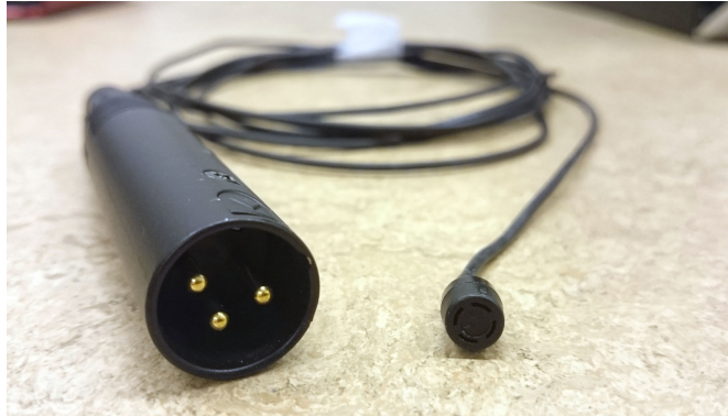
Figure 3.6: AKG C417 condenser microphone with AKG MPA III phantom adapter.
