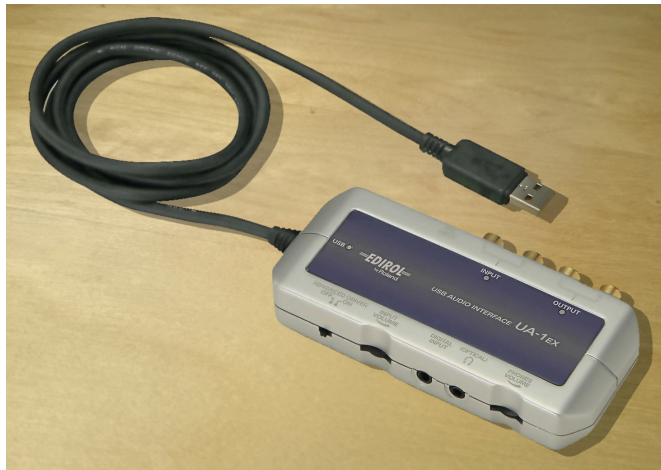
Figure 3.7: Roland UA-1EX audio interface used when recording using the table microphone.
