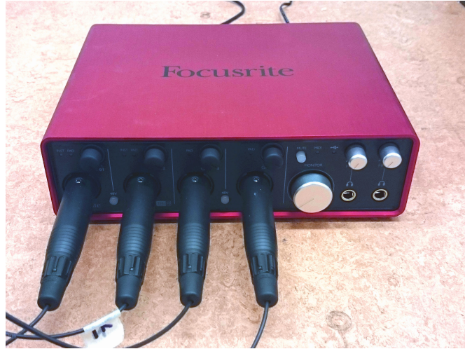
Figure 3.8: Focusrite Scarlett 18i8 USB 2.0 audio interface used when recording in 4-channels using the AKG C417 condenser microphones.
