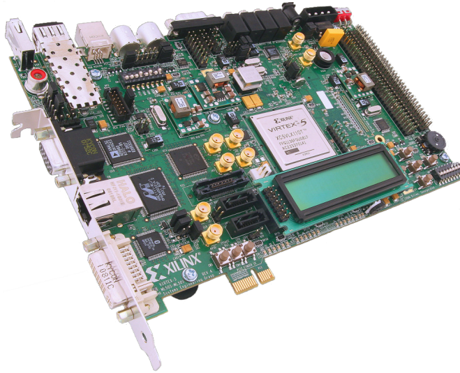
Fig. 6.1: Xilinx XUPV5-LX110T Evaluation Platform with Xilinx Virtex 5 XC5VLX110T FPGA. [9]
