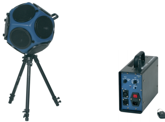
(a) Norsonic Dodecahedron Loudspeaker Nor270H. (b) Norsonic Power Amplifier Nor280.
