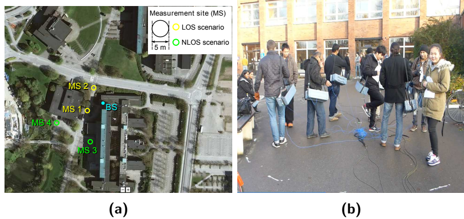
Figure 2.3: UCA with 9 synchronized users - outdoor measurement (a) The measurement area, (b) The users moving randomly in a 5 m diameter circle.
