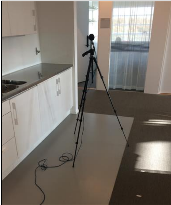
Figure 4.1. Microphone during sound pressure level measurements.
