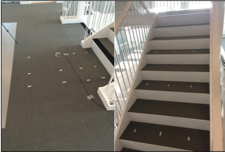
Figure 4.13. Setup during impact hammer test with marking for hitting points.
