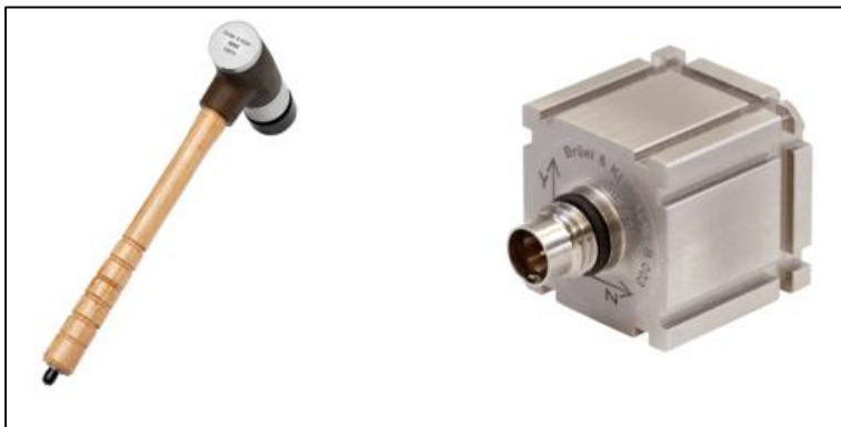
Figure 2.6. An impulse hammer (left) used for exciting vibrations and an accelerometer (right) for collecting the vibration data (Copyright © Brüel & Kjær).
