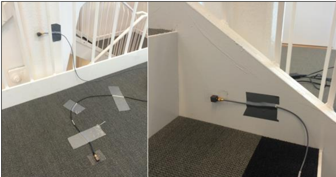
Figure 4.31. Placements of accelerometers. Left; accelerometer on column and slab. Right; accelerometers on stringer.
