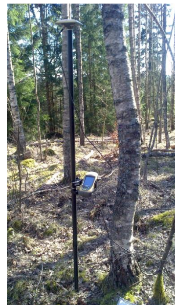
Figure 7. The Topcon GRS-1 and the external antenna attached to a 2 m carbon pole.
